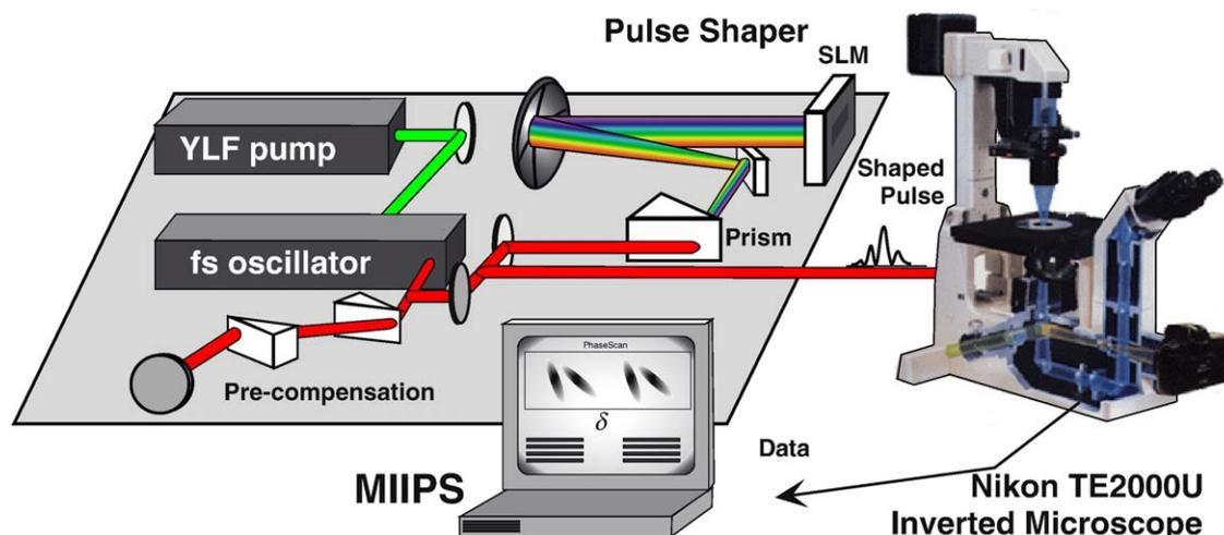
Fig 1. Schematic diagram of experimental setup for two-photon imaging.
