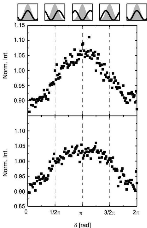
Fig. 3. Femtosecond LIBS dependence on sinusoidal phase functions across the incident pulse bandwidth recorded for Al and Cu samples. The corresponding phase functions as a function of  $\delta$  are shown in the upper insets and  $\delta = \pi$  resembles positively chirped pulses while  $\delta = 0$ ,  $2\pi$  resembles negatively chirped pulses.
