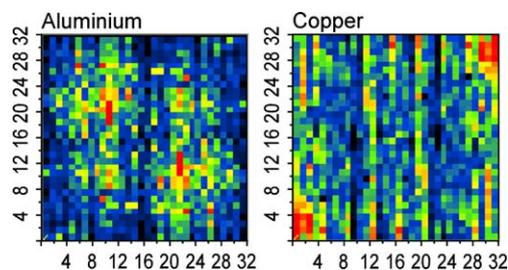
Fig. 4. Femtosecond LIBS dependence on binary phase functions recorded on Al and Cu samples. The data is represented in a 3D map. A rainbow color scheme is used to indicate intensity, with black and blue being the lowest values and red the highest. (For interpretation of the references to color in this figure legend, the reader is referred to the web version of this article.)
