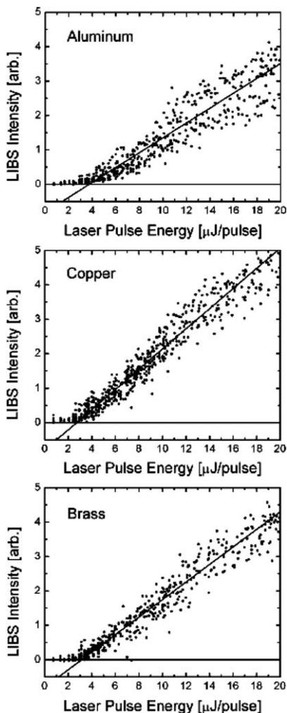
Fig. 1. Femtosecond LIBS laser power dependence recorded for Al, Cu and Brass at 396.152, 521.820 and 481.053 nm, respectively.
