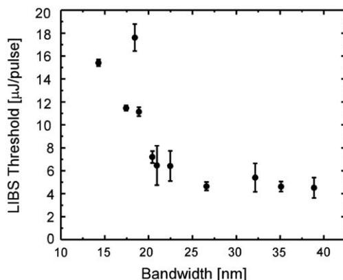
Fig. 5. Femtosecond LIBS threshold dependence on the bandwidth of the pulse (full-width at half maximum). Each data point is the average of three power dependence measurements.
