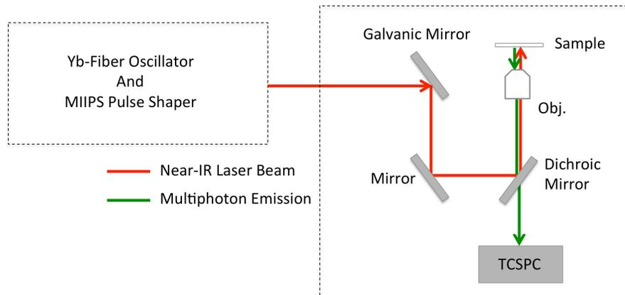
Fig.1. The experimental apparatus consists of an ultrafast fiber laser operating at 1.07  $\mu\text{m}$ , a MIIPS pulse shaper, laser scanning microscope, and a time-correlated single photon counting (TCSPC) detector.
