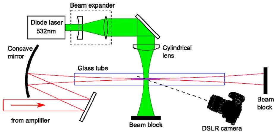
Fig. 1. Experimental setup. Green diode laser is used to create a laser sheet in the vertical plane. DSLR camera images green scattered light from seed particles, unveiling the fluid flow resulting from filamentation in a narrow glass tube.
