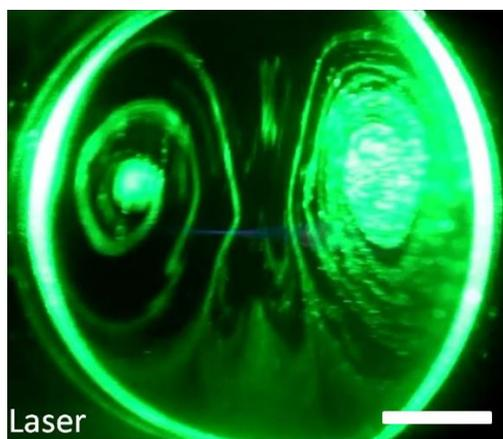
Fig. 3. Vortex pair formed in the glass tube with 14 mm in diameter created by laser filamentation. The filament can be observed as a faint purple hue in the middle of the image. The scale bar is 3mm. Video uploaded as ([Media 2](#)).
