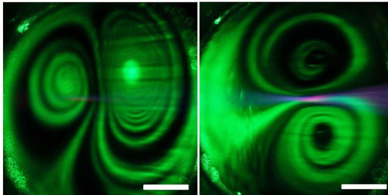
Fig. 2. Two different vortex pairs observed in the 4 mm diameter glass tube induced by laser filamentation. The laser filament is observed as a purple hue in the middle of each image. Scale bars are 1 mm. The number of vortices as well as their relative orientation depends on the position of the laser filament relative to the center of the tube. Video uploaded as [\(Media 1\)](#).
