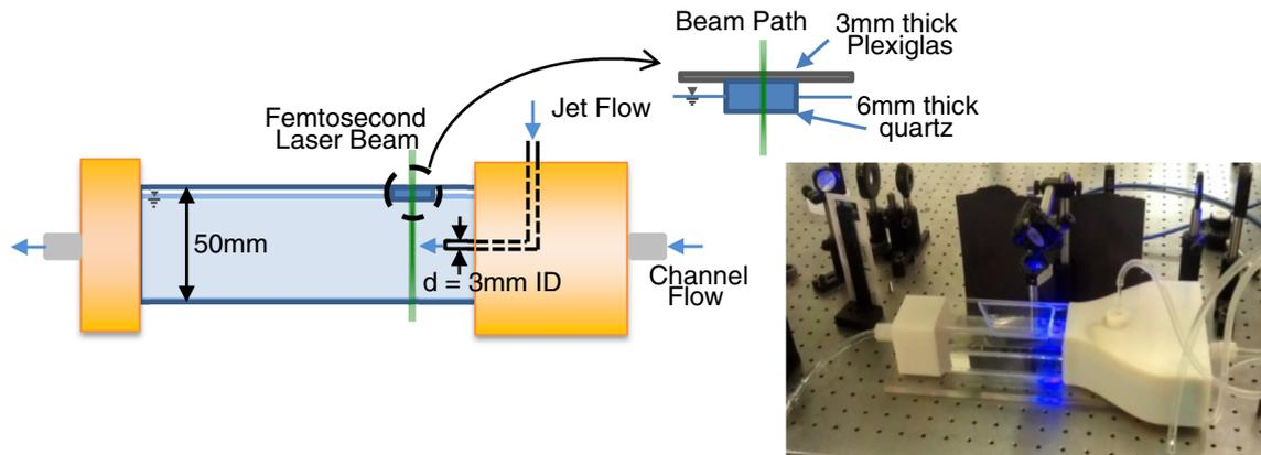
**Fig. 2** Experimental setup for FemtoMTV measurements
