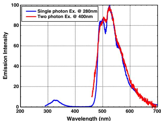
**Fig. 1** Emission spectra for MTV triplex excited by 280 nm (single-photon) (Hu et al. 2006) and 400 nm (two-photon) wavelengths
