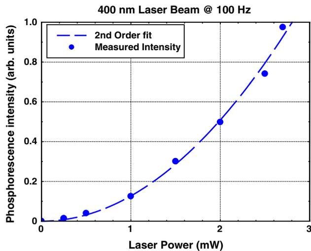
**Fig. 5** Energy dependence of phosphorescence intensity of MTV triplex with two-photon excitation
