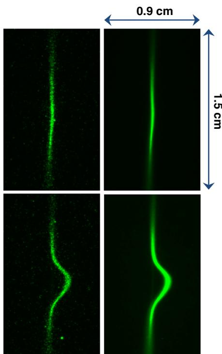
**Fig. 3** Sample instantaneous (*left*) and average (*right*) MTV image pairs of jet flow ( $x/d = 4$ ) with two-photon excitation. *Top* 100  $\mu$ s after laser pulse (400  $\mu$ s exposure), *bottom* 2.6 ms delay after first image (800  $\mu$ s exposure)
