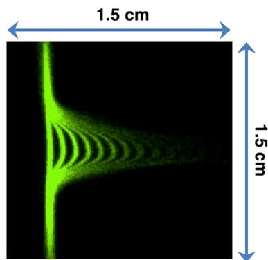
**Fig. 6** Single frame illustrating kHz tagging by the femtosecond laser. Part of a time series video obtained at 10 frames/s
