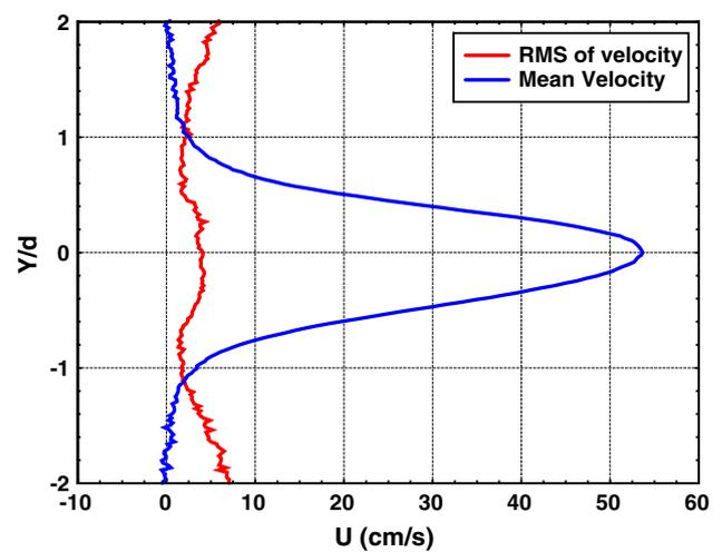
**Fig. 4** Mean and RMS of jet flow velocity measured by MTV using two-photon excitation ( $x/d = 4$ )
