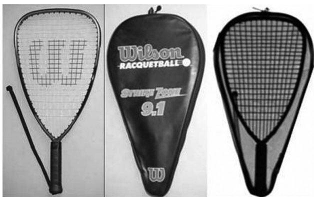
Figure 9 (Left) Photograph of racketball bat. (Middle) Photograph of racketball bat in case. (Right) Terahertz image of racketball bat in case (X.-C. Zhang & Xu, 2009).
