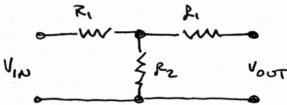
$$R_1 = R_0 \frac{\alpha - 1}{\alpha + 1} = R_0 \frac{0.413}{2.413} = 0.171 R_0$$
