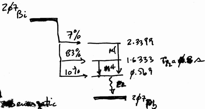
(b) The 1064  $\gamma$  is M4, slow and highly converted into monoenergetic electrons.  $E(e^-) = E_\gamma - BE(e^-)$
