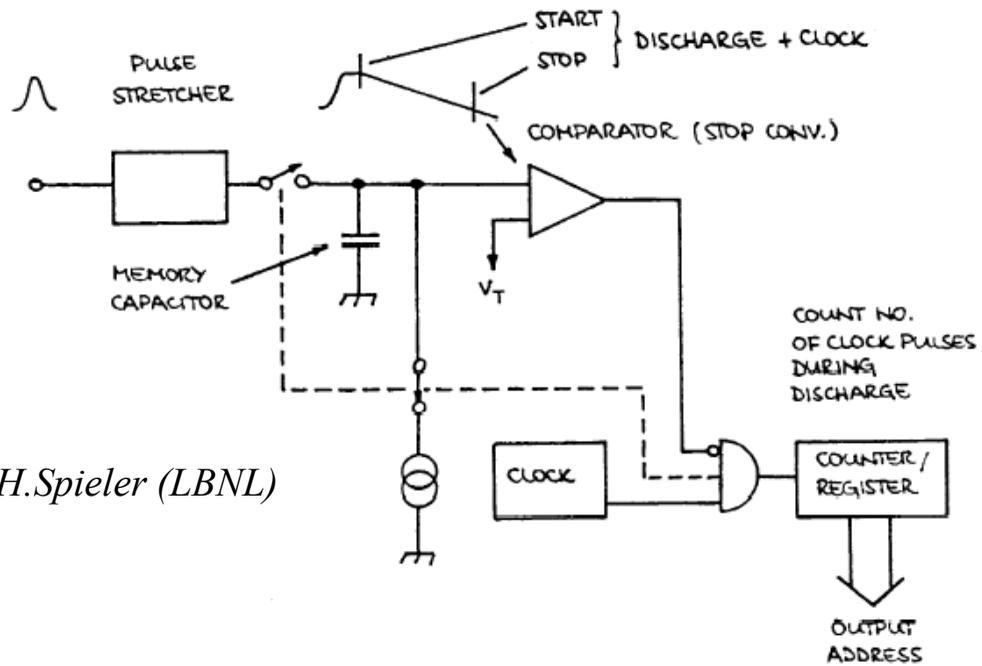
The input signal is stored as a charge on a capacitor that is discharged by a constant current source with a clock (100 up to 400 MHz)
