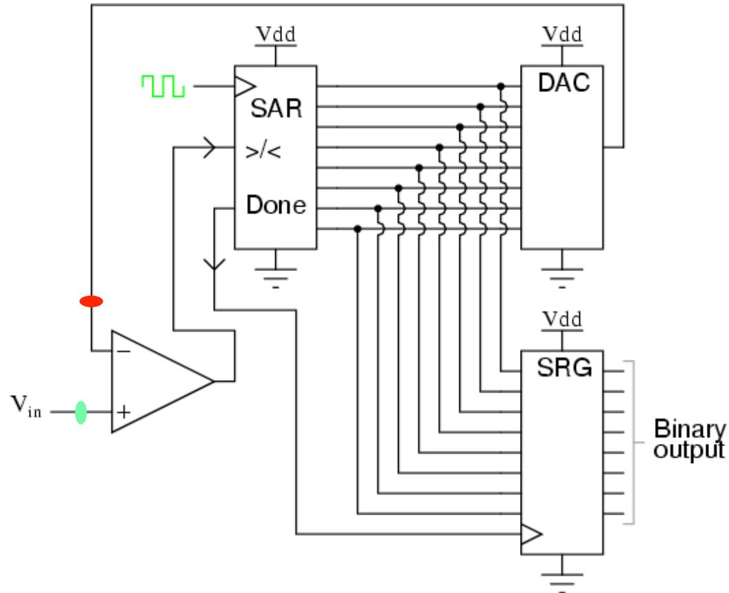
A successive-approximation ADC compares the input signal to a digitally generated signal starting at the midpoint of the range.
