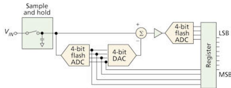
Alternate device determines the upper range and then subtracts it away with a DAC signal ... 15 comparators in each flash ADC to process the signal compared to  $2^8$  comparators in an 8-bit flash ADC.
