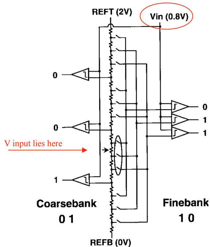
A sub-ranging ADC compares the input signal to the voltage on a resistor chain using several banks of comparators in sequence.
