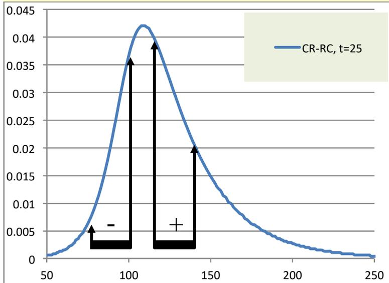
$$Trace_i = \left(\frac{Q}{C}\right) \frac{1}{1 + e^{[-(t_i - t_0)/a]}} \left(\frac{t_i}{\tau}\right) e^{-t_i/\tau}$$
