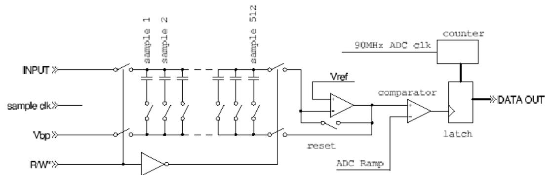
Switched Capacitor Array & ADC (SCA)
