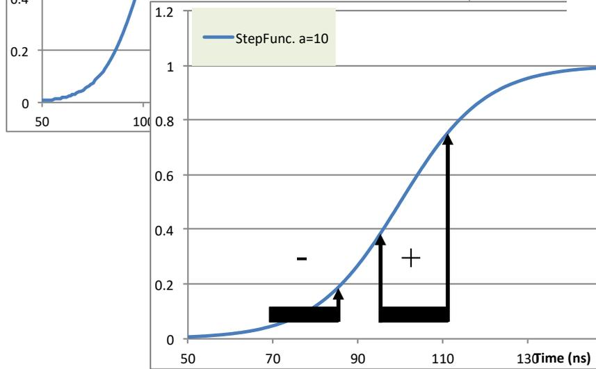
$$Trace_i = \left(\frac{Q}{C}\right) \frac{1}{1 + e^{-(t_i - t_0)/a}} \quad t_0 = 100ns, a = 10ns$$
