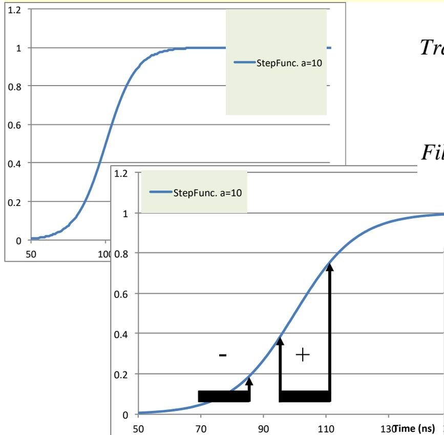
$$Trace_i = \left(\frac{Q}{C}\right) \frac{1}{1 + e^{-(t_i - t_0)/a}} \quad t_0 = 100ns, a = 10ns$$
