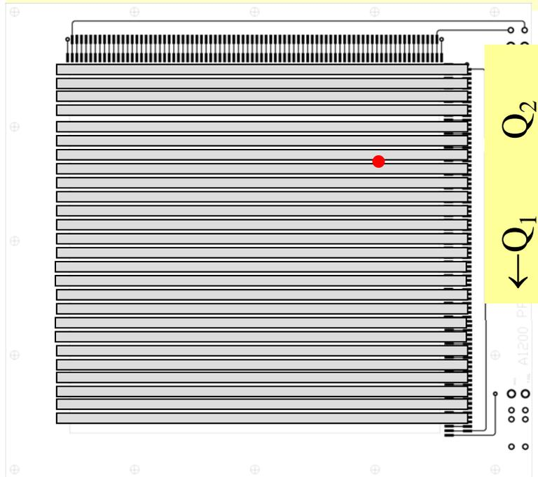
Conventional: resistor chain, two linear channels
