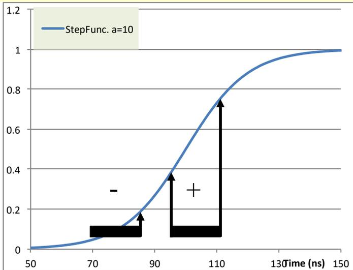
$$Trace_i = \left( \frac{Q}{C} \right) \frac{1}{1 + e[-(t_i - t_0) / a]}$$
