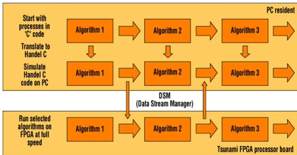
Accelerating a C-based algorithm involves translating the code to Handel-C, simulating the Handel-C design on a PC, and then running the design on an FPGA processor.
