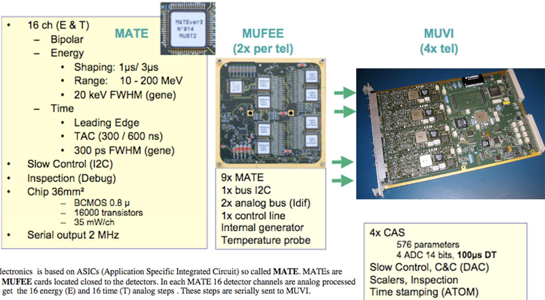
MUST2 Electronics is based on ASICs (Application Specific Integrated Circuit) so called **MATE**. MATEs are housed on **MUFEE** cards located closed to the detectors. In each MATE 16 detector channels are analog processed in order to get the 16 energy (E) and 16 time (T) analog steps. These steps are serially sent to MUVI.
