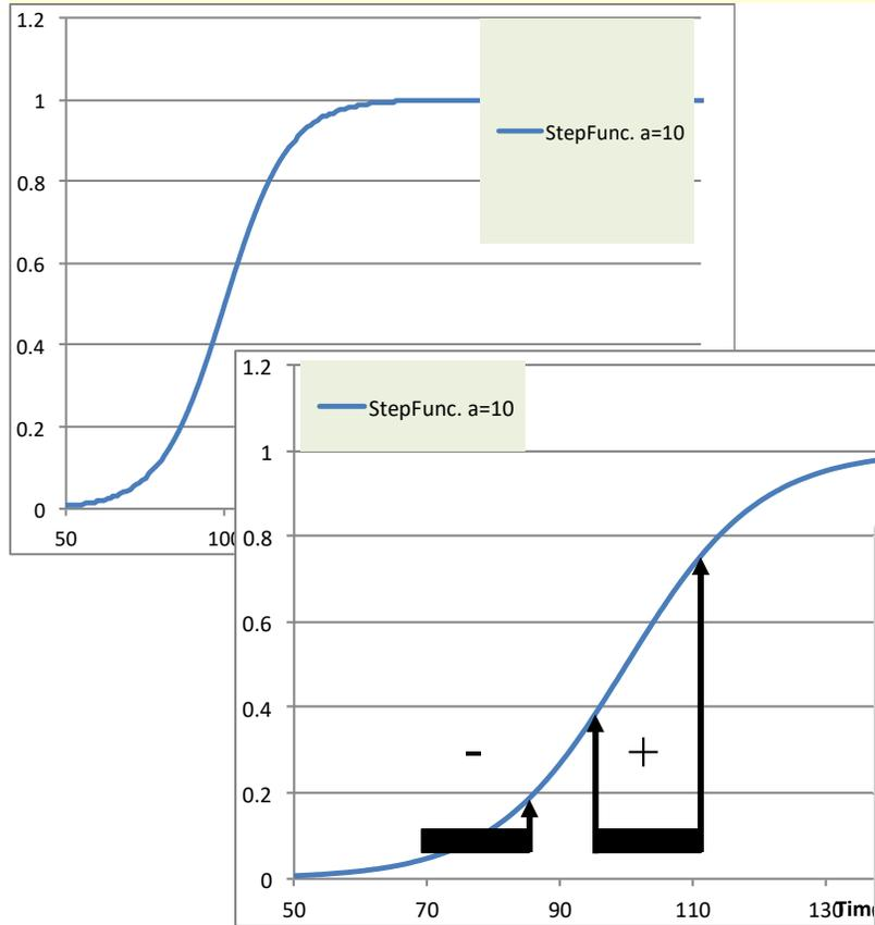
$$Trace_i = \left(\frac{Q}{C}\right) \frac{1}{1 + e^{[-(t_i - t_0) / a]}} \quad t_0 = 100ns, a = 10ns$$
