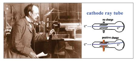
FIGURE 1: J. J. Thomson and a cathode ray tube used to perform some of the first m/z measurements. Deflection of the electron was observed once the electric field was turned on.
