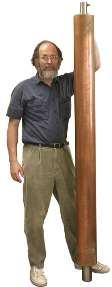
Large Chalk River \text{BF}_3 neutron Proportional Counter (ca. 1960)
