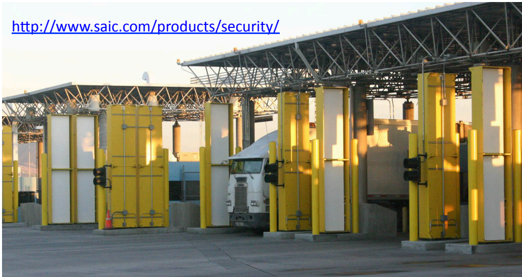
A truck passes through an Advanced Spectroscopic Portal before a security booth at a Container Terminal in Staten Island, N.Y., April/2007.
