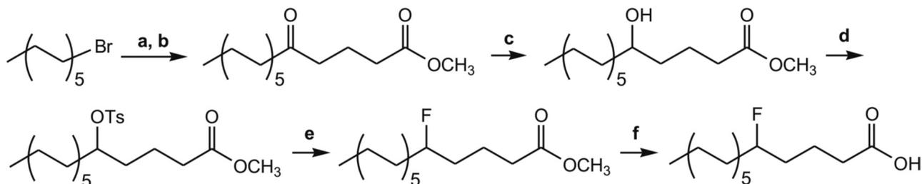
Scheme 1. Synthesis of 5-<sup>19</sup>F-palmitic acid.
