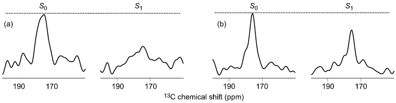
**Fig. S3.** (a)  $^{13}\text{C}$ - $^{31}\text{P}$   $S_0$  and  $S_1$  spectra of a sample containing HFPmn-A21 and (b)  $^{13}\text{C}$ -( $5$ - $^{19}\text{F}$ ) spectra of a sample containing HFPmn-L9. The dephasing time was (a) 32 ms or (b) 24 ms. All spectra were processed with 200 Hz Gaussian line broadening and polynomial baseline correction. Each spectrum was the sum of (a) 50,000 or (b) 20,000 scans.
