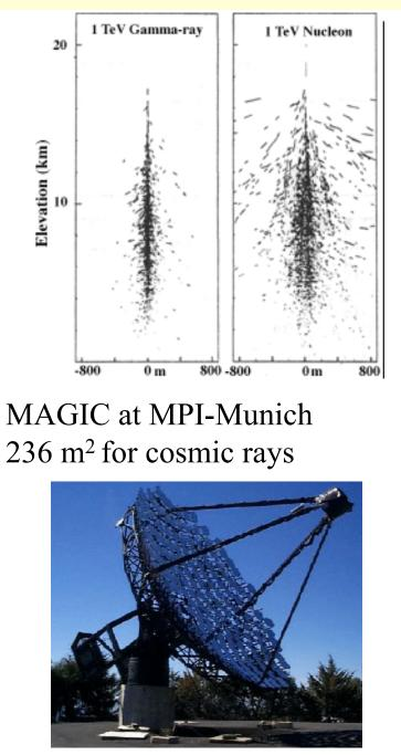
Extremely high energy  $\gamma$ -ray from space pairproduces at the top of the atmosphere and creates a characteristic shower of secondaries.
