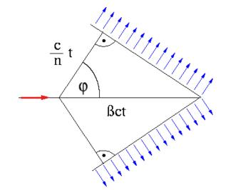
n is the dielectric refractive index,  $\alpha = 1/137$ x is the path length in radiator e<sup>-</sup>~390 photons/cm in water (at 300-700 nm)
