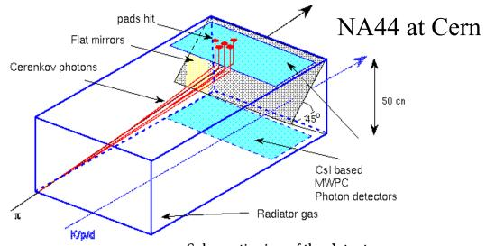
Schematic view of the detector
