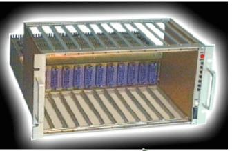
NIM (nuclear instrumentation module): Nuclear Physics standard container/voltages/ power
