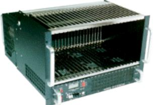
CAMAC (computer automated measurement and control): Nuclear Physics standard container/voltages/power Computer bus (back plane) with [86 lines] Address lines / write / read (24b) / control lines Bus speed 1 MHz .. Geographic: "BCNAF" "LAM"
