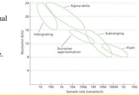
Typical nuclear physics pulsed device 12b /10  $\mu s \sim 10^7$  b/s
