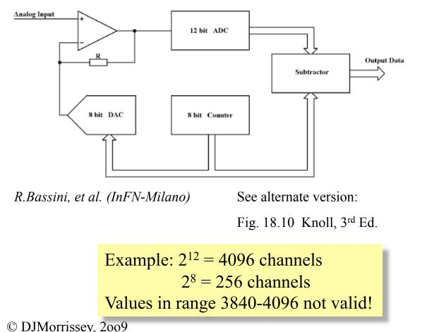
The counter contains a random number and generates a voltage that is added to the input voltage.
