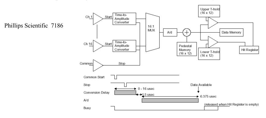
•Counting clock pulses between start/stop signals – generally limited to Dt =1ns or lower resolution, can read multiple hits before & after start (with appropriate logic)
