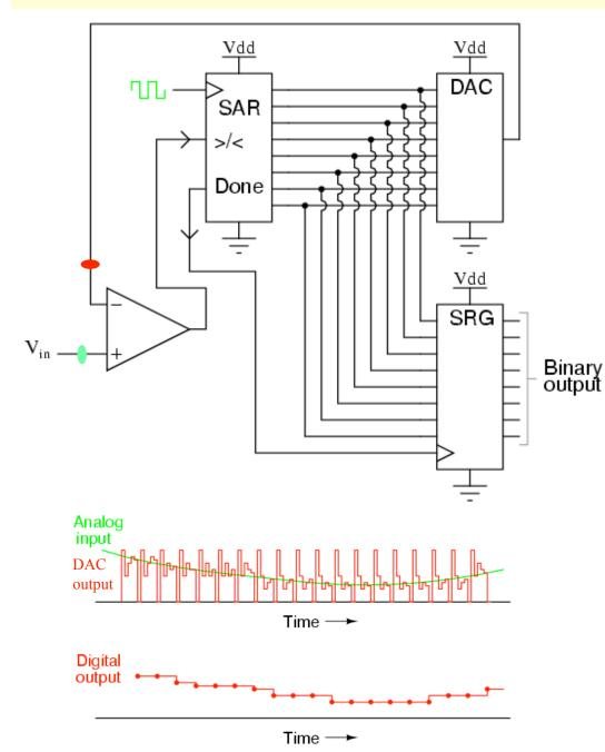
A successive-approximation ADC compares the input signal to a digitally generated signal starting at the midpoint of the range.
