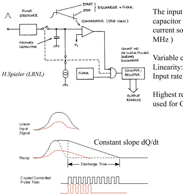
The input signal is stored as a charge on a capacitor that is discharged by a constant current source with a clock (100 up to 400 MHz )
