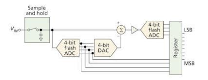
A sub-ranging ADC compares the input signal to the voltage on a resistor chain using several banks of comparators in sequence.
