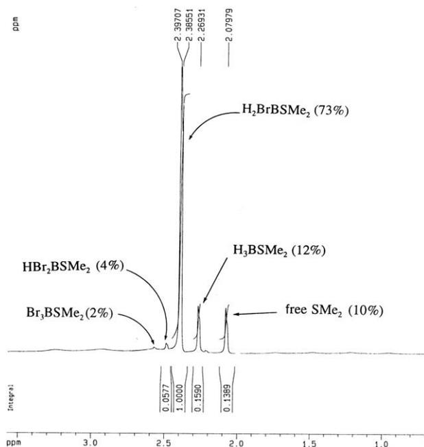
**Figure 2** <sup>1</sup>H NMR spectrum of a sample of BH<sub>2</sub>Br·SMe<sub>2</sub> purchased from Aldrich Chemical Co.
