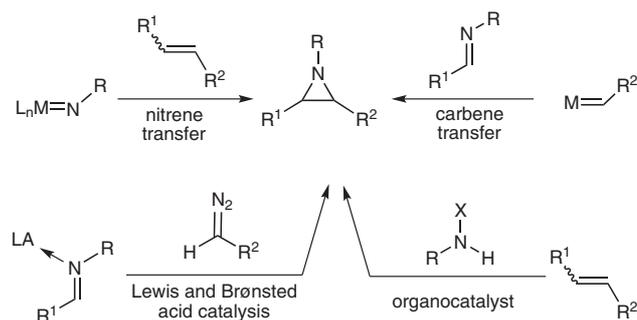
**Scheme 1** Four approaches for catalytic AZ reactions
